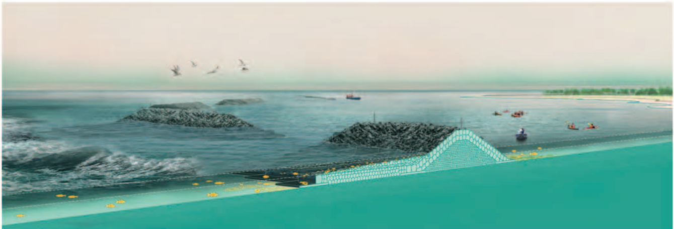
Fig. 7 Section of proposed living breakwater coastal condition. Image courtesy of Scape Studio.
